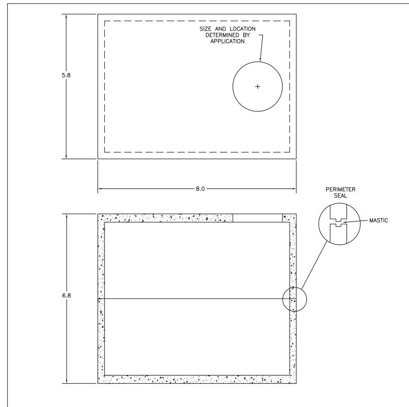
NOTE: 0.27 THICK WALLS 0.33 THICK TOP and BOTTOM NOT TRAFFIC RATED
